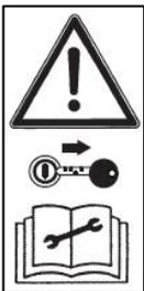
operations on the machine, stop the engine, take out the ignition key and follow the instructions in the manual.
