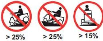
Be care when operating the lawnmower near drop-offs, ditches or embankments
