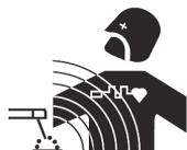
The electric currents flowing through a conductor cause electrical and magnetic fields (EMF). The welding current generates an EMF field around the welding circuit and the welding equipment.
