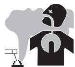
The fumes, gases and dust produced during welding are hazardous. It is mandatory to ensure adequate ventilation and/or extraction to keep fumes and gases away from the work area. An air fed helmet is recommended in cases of insufficient air supply in the workplace.
